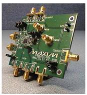
Objective: For this dual-band triple-mode front-end IC, to experimentally tune for the best-possible cellular LNA linearity available in CDMA low-gain high-linearity mode.
